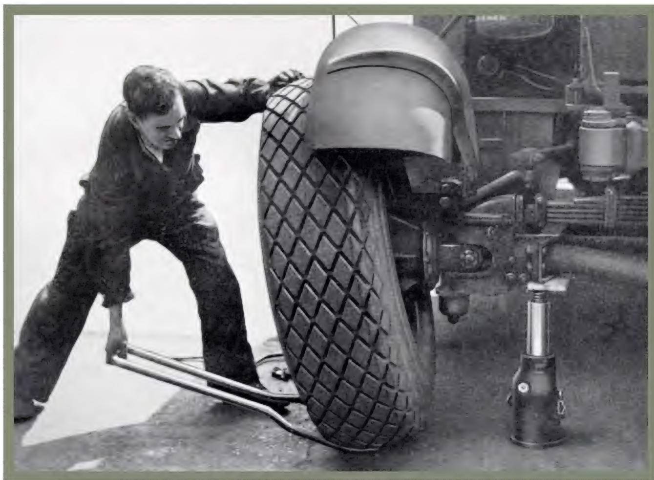
● Despite their considerable weight, it was possible for one man to remove a wheel and tyre using a double-pronged crowbar.
