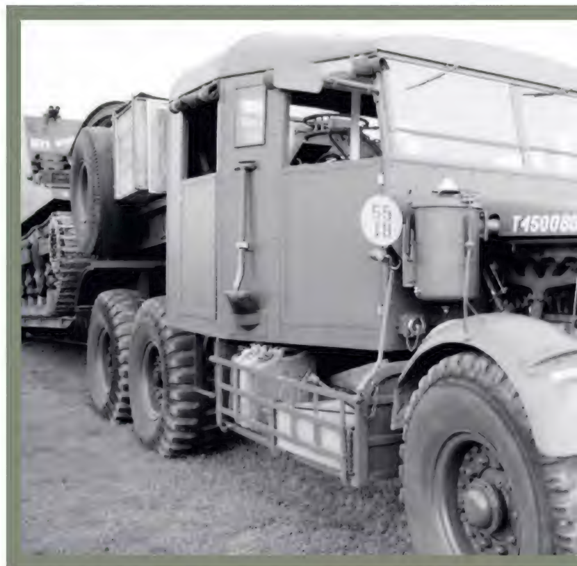
● Looking a little tired and cobwebby around the wheels, this tank transporter was photographed at the REME Museum. The side lights and the lower headlights are later additions.
