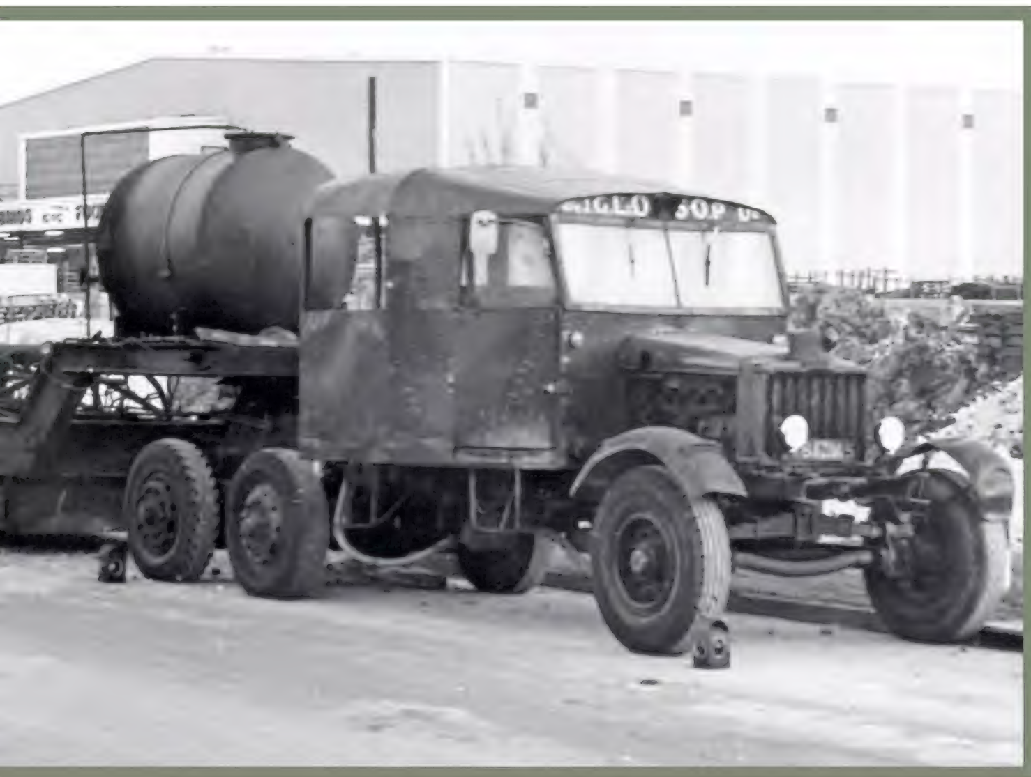
● Extensively-repanelled 30-ton tractor, proudly wearing a 'Scammell' badge on the roof panel. Note the sliding cab window... real luxury for the Pioneer driver!
