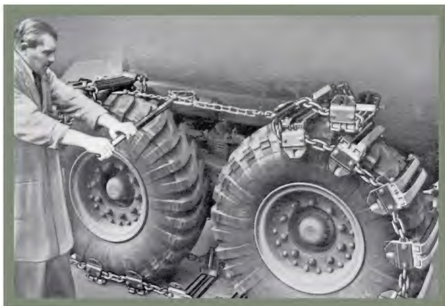
● Fitting and tensioning the Kennedy & Kemp caterpillar tracks to the rear wheels. Often described as 'chains', the tracks were intended to improve traction on soft ground or in ice and snow.
