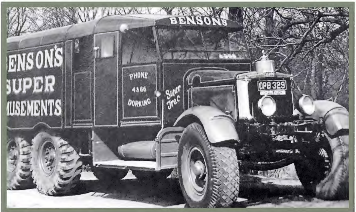
● Nicknamed 'Challenger', this tractor belongs to Bensons Super Amusements of Dorking. At a glance it more closely resembles the R100 artillery tractor, but the length of the wheelbase and the cab extension give the game away. Note how the air tank for the brakes has been moved from behind the cab into the stowage basket.
