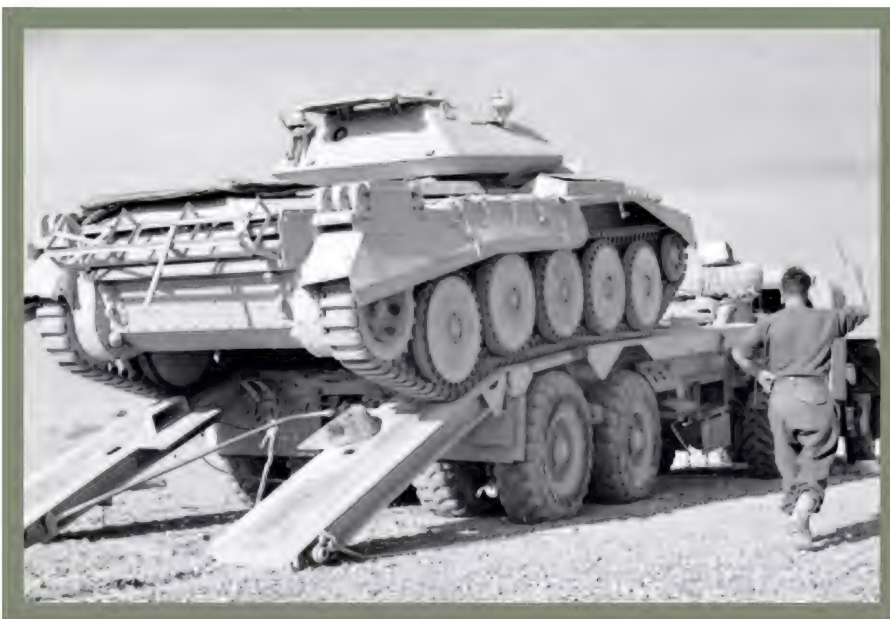
● With the semi-trailer ramps lowered, this 30-ton Pioneer waits while an A15 Crusader cruiser tank climbs on board. Note the guide shoes, or buttresses, on the ramps to help keep the tank running straight, but note also that the crew has not deployed the stabilising jacks.
