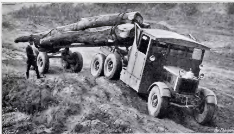
● These illustrations are taken from 'The Engineer' magazine, January 1932. The upper photograph shows how the Pioneer dwarfs an Austin Seven motorcar, whilst the lower picture, taken at the MWEE test facility at Bagshot, shows a Pioneer carefully picking its way over rough ground, loaded with several tons of round timber masquerading as pipeline sections.
