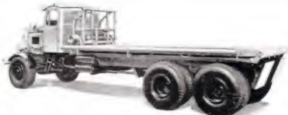
"CONSTRUCTOR" 6-wheel drive 21' 9" Wheelbase Full Oilfields Truck. Fitted with winch, tail roller, headache rack and gin poles. Load capacity 40,000 lbs.
