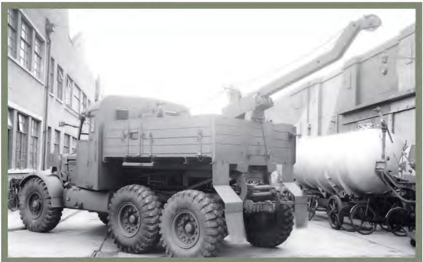
● Pioneer SV/2S breakdown-recovery tractor with the jib at full extension. In this position, the jib was rated for a lift of 2 tons (2.04 tonne); in the inner position, the rating was 3 tons (3.06 tonne).
