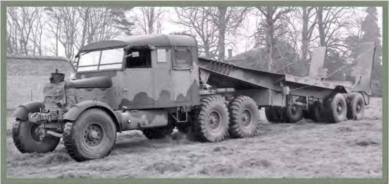
● Resplendent in disruptive camouflage, consisting of a background green colour, with the pattern applied as areas of black or very dark grey, this early 30-ton outfit shows the steep angle to the deck of the semi-trailer, and the long loading ramps. Note, particularly, the radiator muff.
