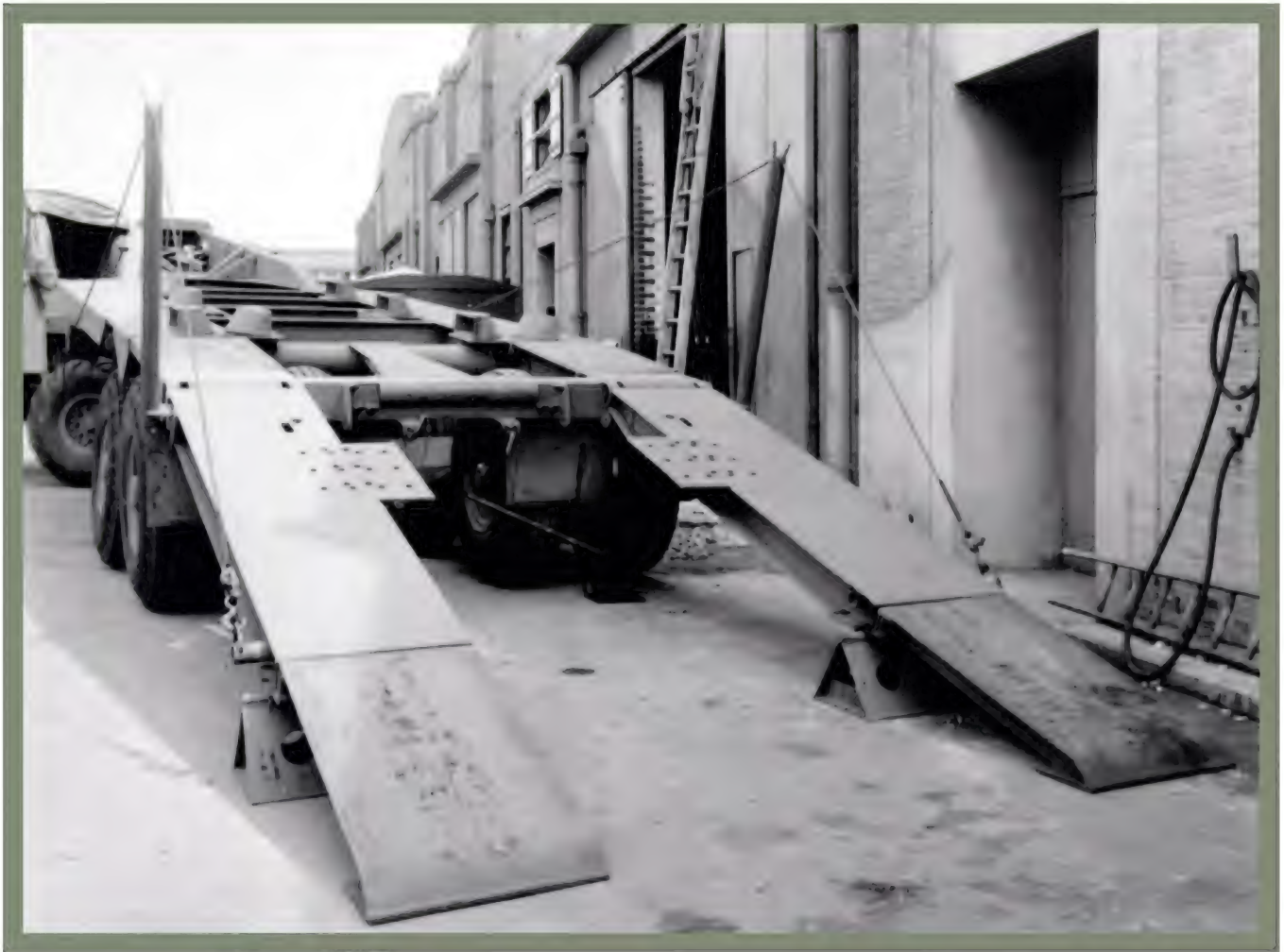
● 30-ton semi-trailer with the ramps in the loading position, with the tubular ramp cable stanchions deployed; a hand winch is provided to raise and lower the ramps, and, when not in use, the stanchions are carried in the stowage locker. The handle of a jack can just be seen behind the right-hand trailer wheels.
