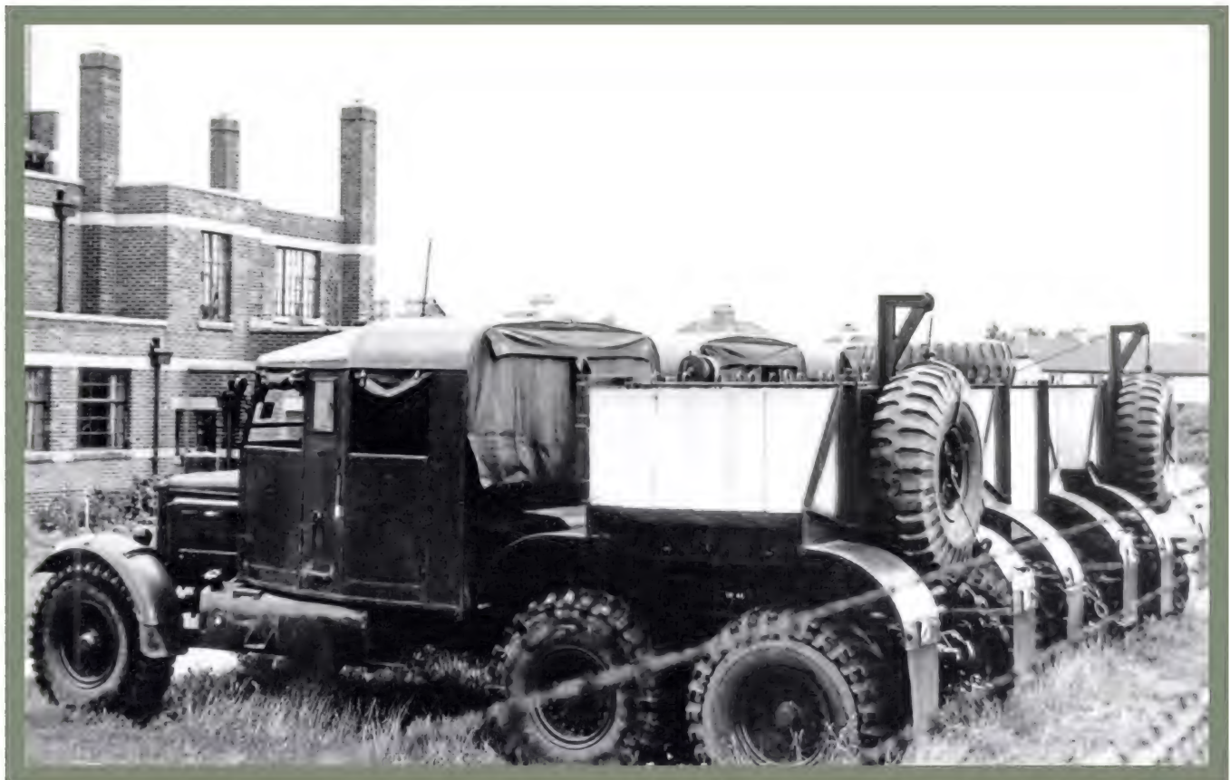
● After WW2 was over, REME used heavy concrete blocks to convert a handful of 30-ton Pioneers into ballast tractors for use with engineer's drawbar trailers by 27 Command Workshop REME. They were described as Pioneer R100/2, but were soon superseded by new Scammell Constructors.
