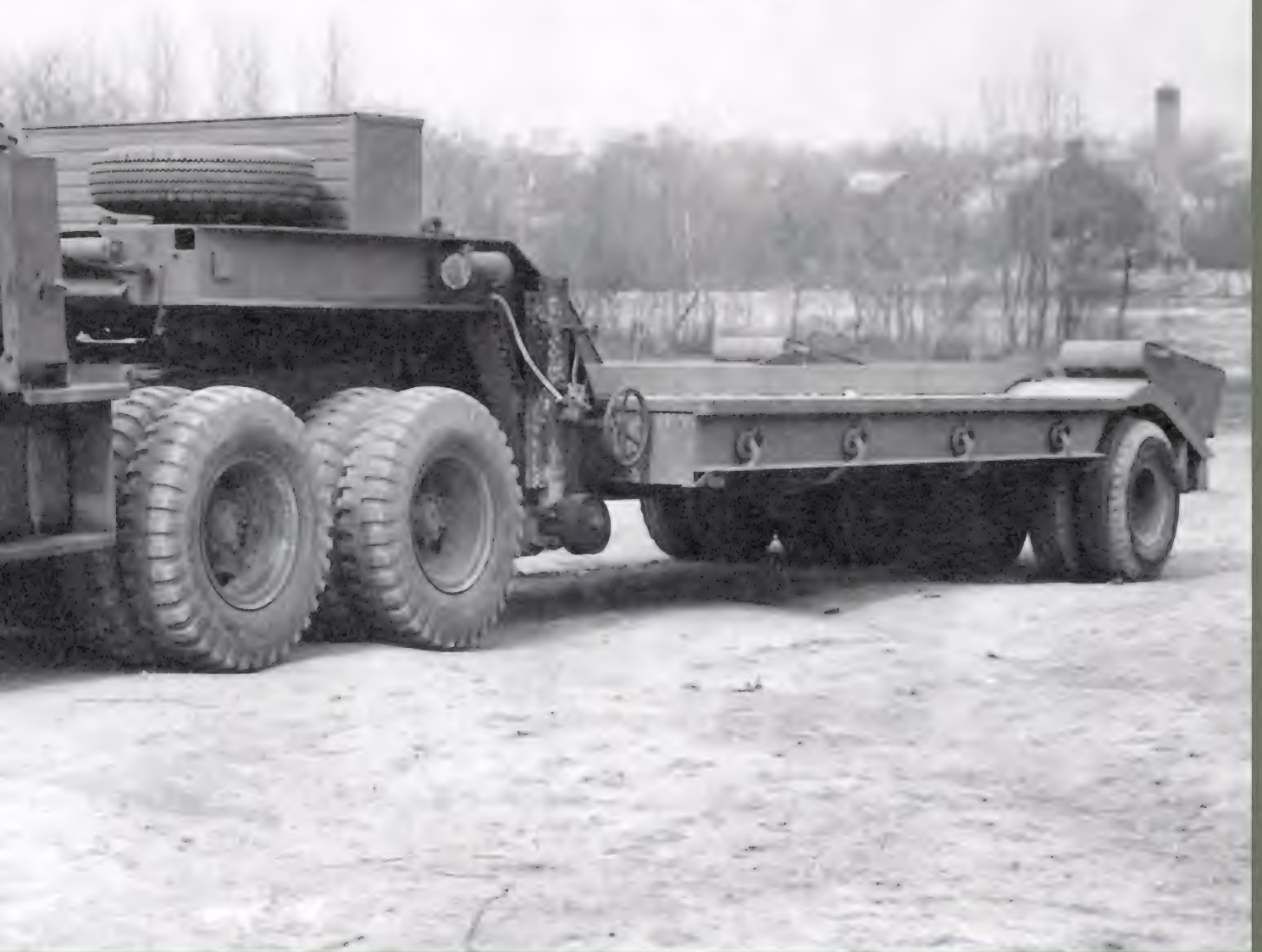
● Rated at 18 tons, the White-Ruxhall 922 was typical of the ex-French contract vehicles that were diverted to Britain in 1940, after the fall of France, and fitted with locally-made bodies to carry light tanks, such as this 19-ton Crusader II, which weighed in at 42,560 lb (19,345kg). Nearly 250 were in service during 1941/42, but they were quickly found to be obsolete in this role and were converted to cargo vehicles.
