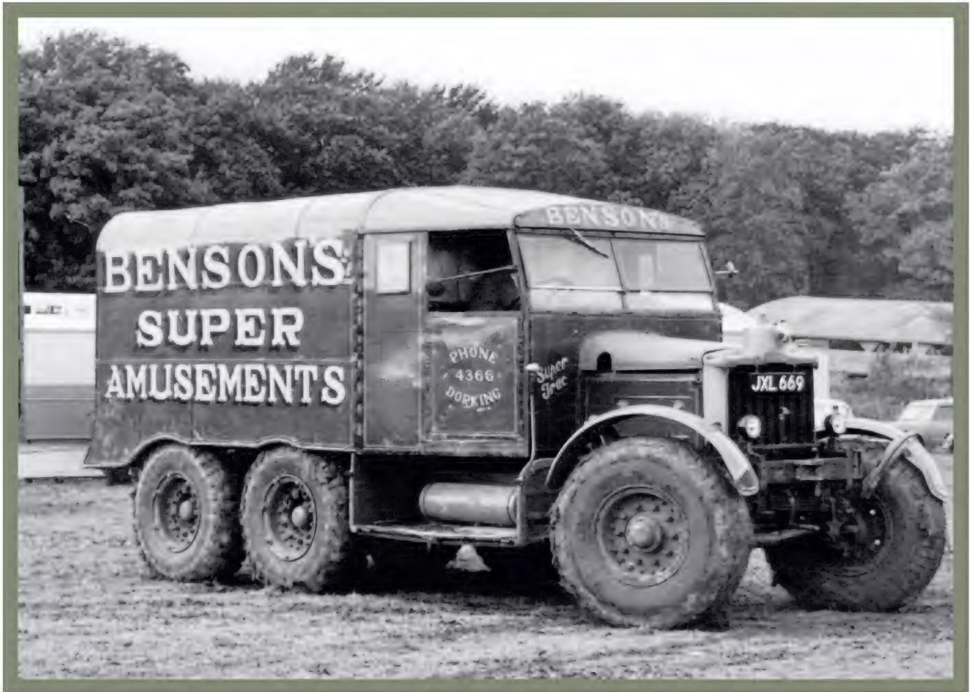
● For comparison, here's another Pioneer, this time an R100 artillery tractor with with a less flamboyant variation of the tail-end treatment already illustrated. Once again, the air receiver for the braking system has been moved to the stowage box, and the front mudguards appear to be longer than normal.
