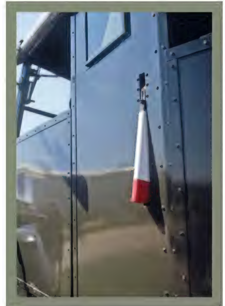
● Red-and-white painted hand-operated semaphore signal... on the left hand side of the tractor only!
