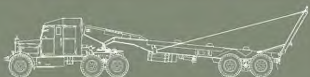
● Side elevation - 30-ton tank transporter (TRMU30/TRCU30) with second, later, pattern of semi-trailer
