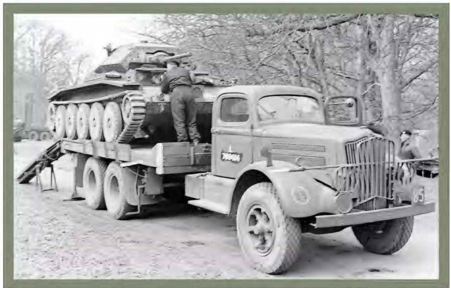
● Also rated at 18 tons, the White 920 was another ex-French contract vehicle, converted to a tank carrier. The load is a Crusader cruiser tank, the flat disk wheels suggesting that it could be the prototype.
