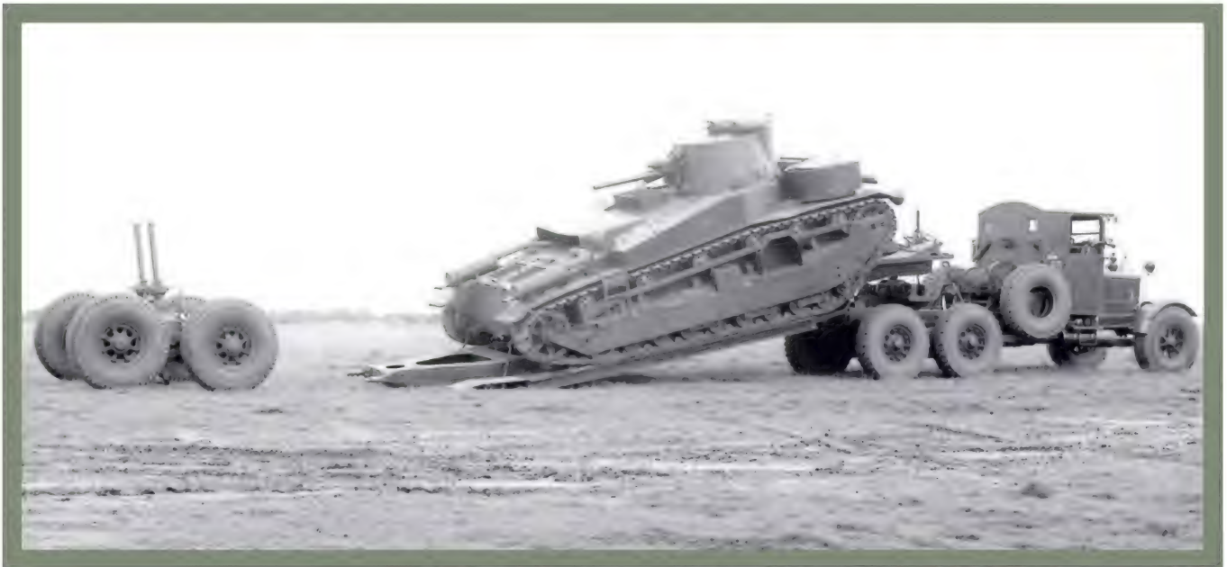
● The first Pioneer tank transporter was supplied in 1932. Rated at a nominal 18 tons, it consisted of a Pioneer tractor, coupled to a low-loading semi-trailer of riveted construction designed to transport the Vickers medium, or similar, tank; in this photograph the tank is a Vickers A6E1. In order to get the tank on board, it was necessary to detach the bogie wheels of the trailer.
