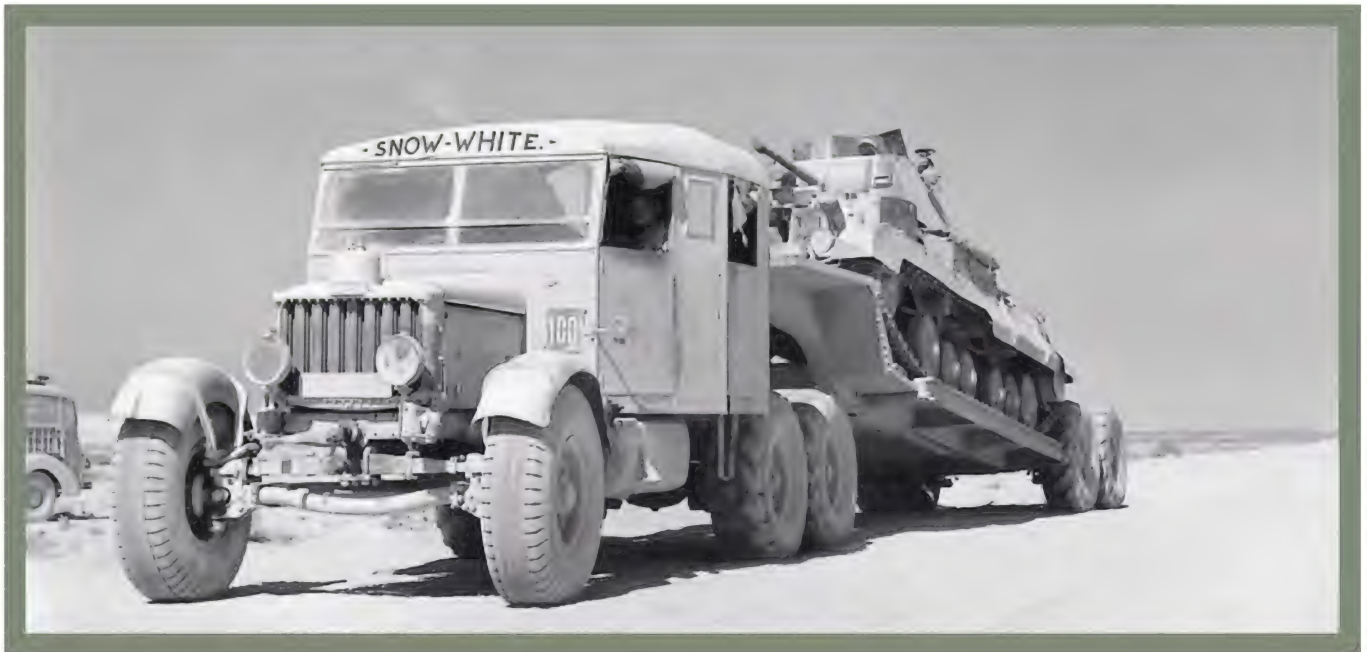
● Early 20-ton Pioneer with the riveted semi-trailer. Like the original 1932 semi-trailer, it was necessary to remove the rear bogie of the semi-trailer to effect loading. Only eight semi-trailers were constructed with this configuration.
