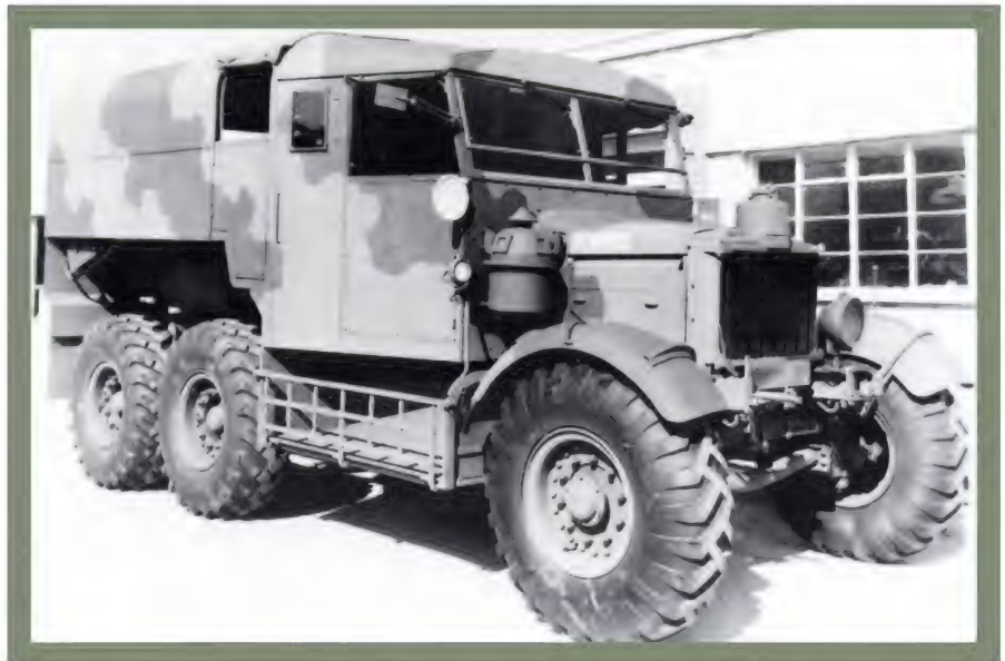
● Early R100 heavy artillery tractor designed for towing weapons such as the 6in and 7.2in howitzers, and the 60-pounder gun. A total of 980 artillery tractors were constructed between 1935 and the end of the war; this example was supplied under contract V3610, dating from 1939.
