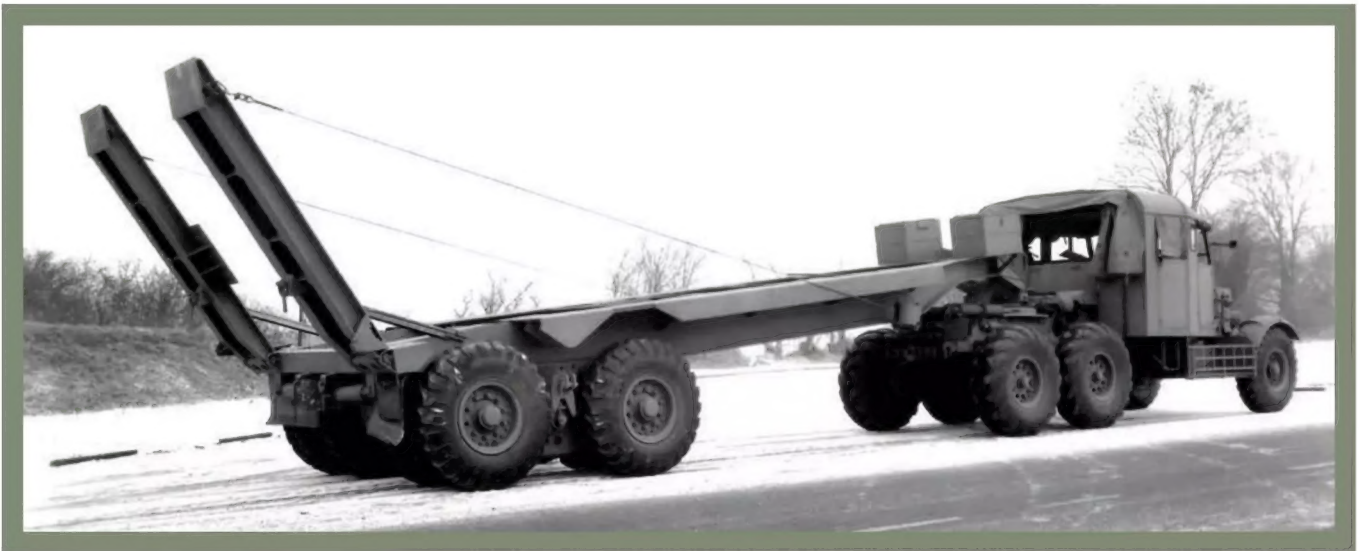
● Early-production 30-ton Pioneer with the original steeply-angled trailer deck. The position of the deck over the fifth wheel created an unacceptable loaded height when carrying the M3 medium tank - the General Lee or the General Grant.
