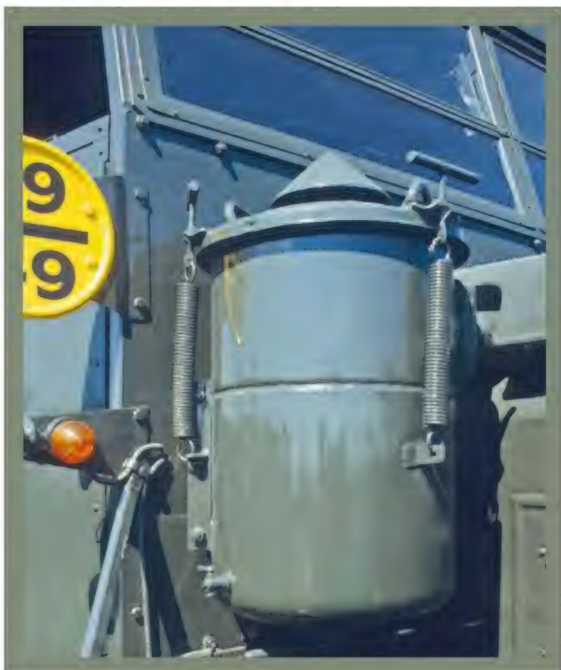
● Two types of engine air filter were used; this is the pressed-steel version. The other was of cast construction.
