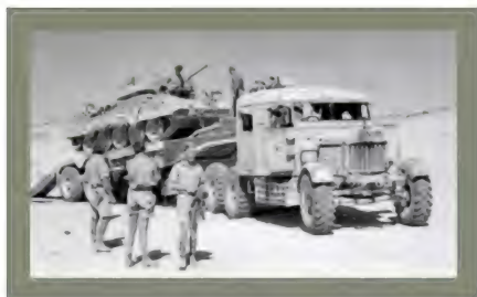
● Charmingly nicknamed 'Molly', this 30-ton Pioneer, with a late trailer, was photographed in North Africa. The load is an A15 Crusader cruiser tank. Note how the windscreen on the tractor has either been opened wide or removed to aid ventilation.
