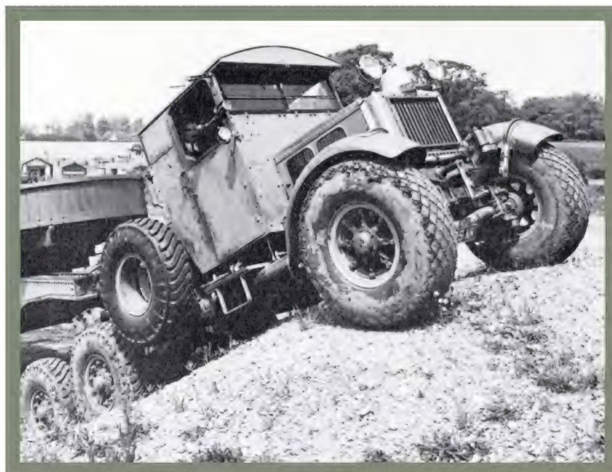
● Towing a low-loader trailer, of riveted construction, on which is loaded a second trailer carrying test weights, giving a total load of 17 tons, this Pioneer demonstrates how it is able to climb a steep bank of loose gravel without difficulty.
