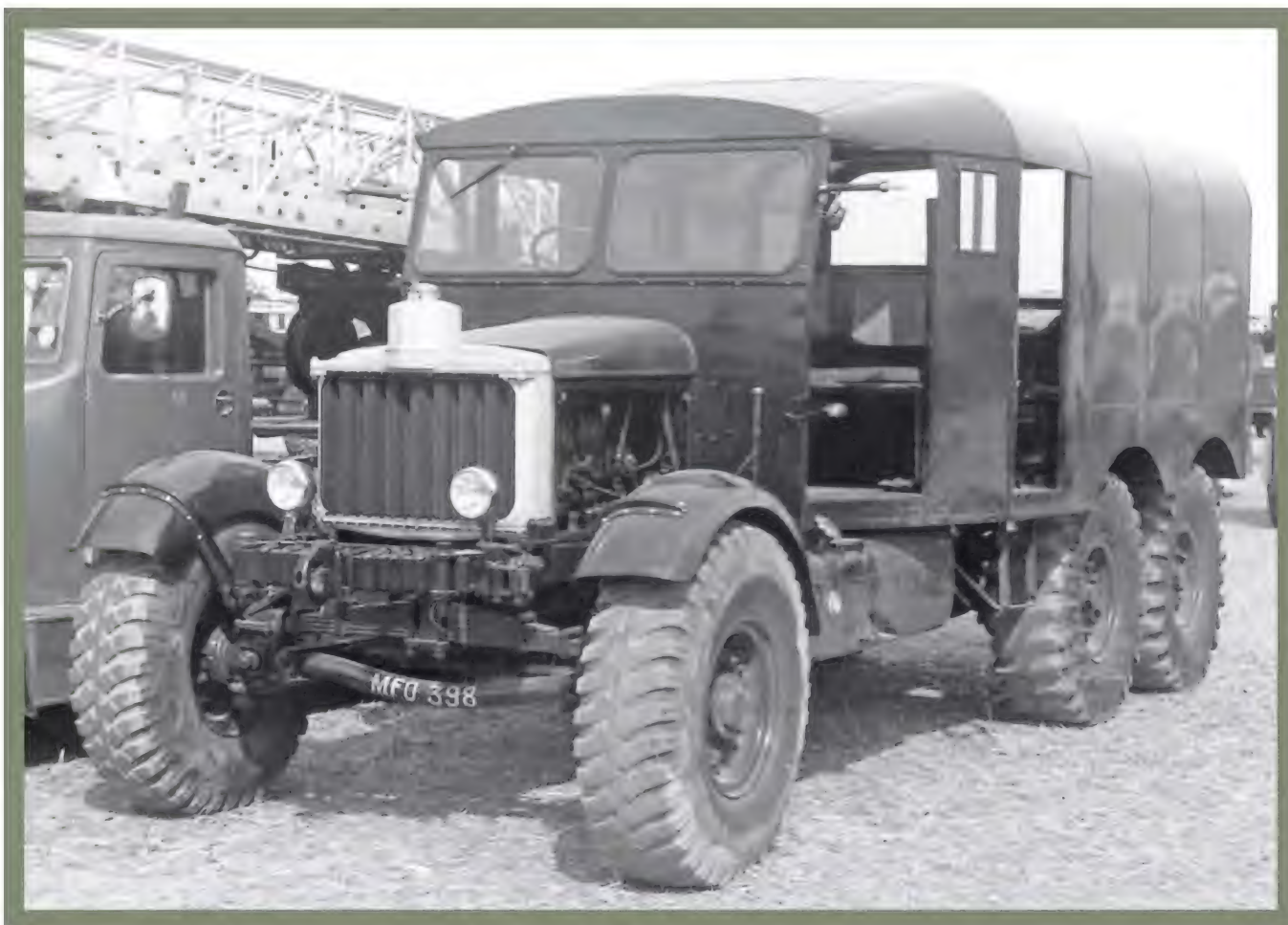
● This is another example of a tank transporter that has been rebodied with what could be considered as a version of the R100 artillery tractor body... the placement of the number-plate is interesting.
