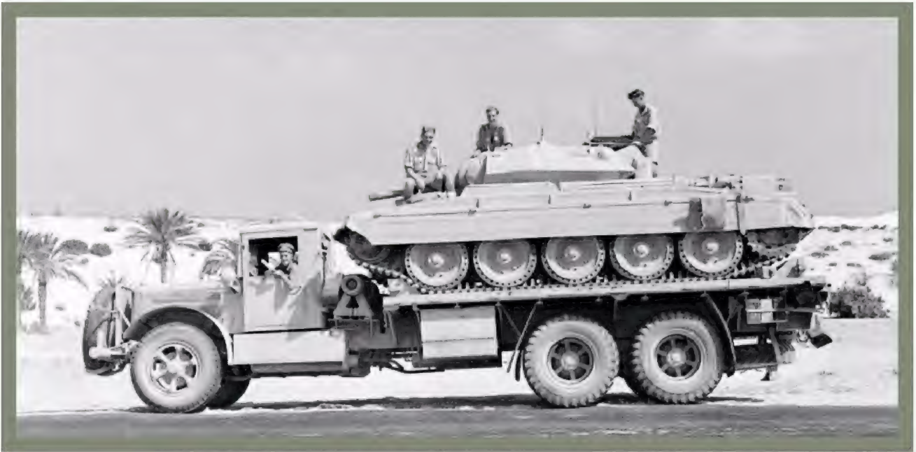
● Rated at 18 tons, the White-Ruxhall 922 was typical of the ex-French contract vehicles that were diverted to Britain in 1940, after the fall of France, and fitted with locally-made bodies to carry light tanks, such as this 19-ton Crusader II, which weighed in at 42,560 lb (19,345kg). Nearly 250 were in service during 1941/42, but they were quickly found to be obsolete in this role and were converted to cargo vehicles.
