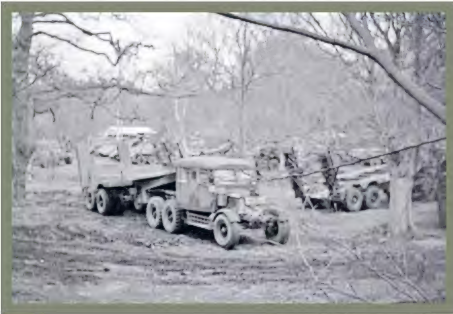
● ABOVE Disabled M4 Sherman medium tank being returned to a workshop for repair on a 30-ton Pioneer, with the late semi-trailer. Disabled tanks were loaded using the Pioneer's on-board winch.
