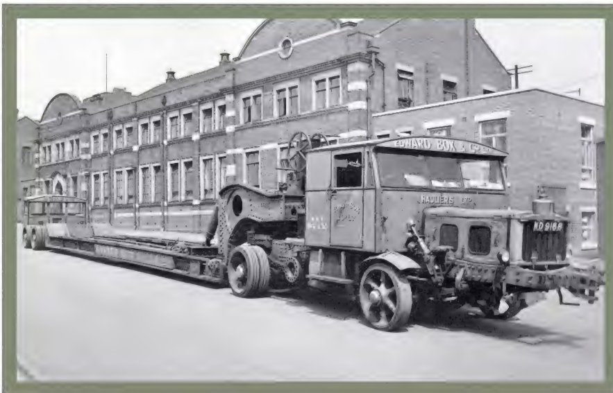
● A rudimentary cab was provided at the rear of the semi-trailer, occupied by a brake and steersman who was in contact with the front cab by means of a sound-powered telephone system.
