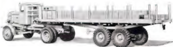
"MOUNTAINEER" 4 wheel drive Motive Unit with Flat Platform Semi-Trailer. Load capacity 56,000 lbs.
