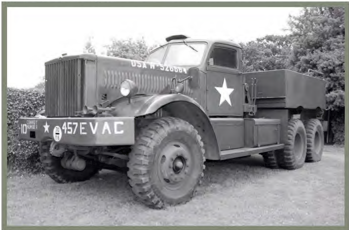
● The appearance of the 40-ton Diamond T tank-transporter train in 1941/42 brought to an end discussions regarding redesigning the Pioneer to accept more weight. The photograph shows the early closed-cab Model 980, which lacked the ability to winch from the front. The air horns and indicators are a wise addition, but are not original.
