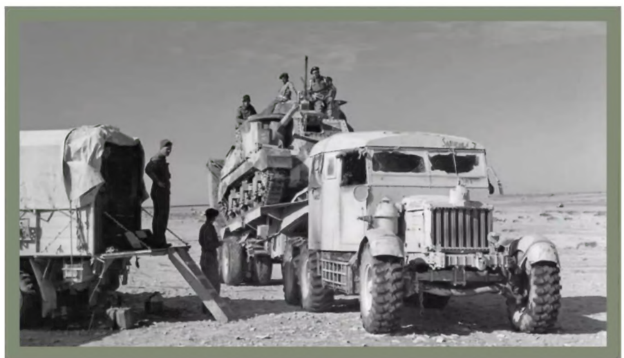
● Sand-painted 30-ton Pioneer and redesigned semi-trailer in the Western Desert, loaded with the US M3 medium tank. The M3 was the first US tank to be constructed in quantity, and, although far from ideal, started to appear in 1942, forming the mainstay of the fighting forces in the Middle East.
