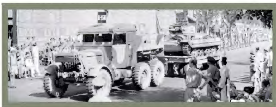
● Pioneer SV/2S breakdown-recovery vehicle acting as a tank transporter with a Valentine infantry tank Mk III on an 18- or 20-ton drawbar trailer.
