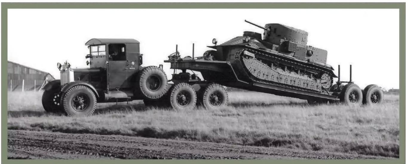
● Rated at 18 tons, and supplied in 1932, the prototype Pioneer tank transporter featured a low-loading trailer of riveted construction, with a removable bogie. It was intended to carry the Vickers medium tank, which had a fighting weight of around 13.5 tons. A handful of these, by then obsolete, tanks fought in the Western Desert.
