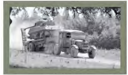
● ABOVE Disabled M4 Sherman medium tank being returned to a workshop for repair on a 30-ton Pioneer, with the late semi-trailer. Disabled tanks were loaded using the Pioneer's on-board winch.
