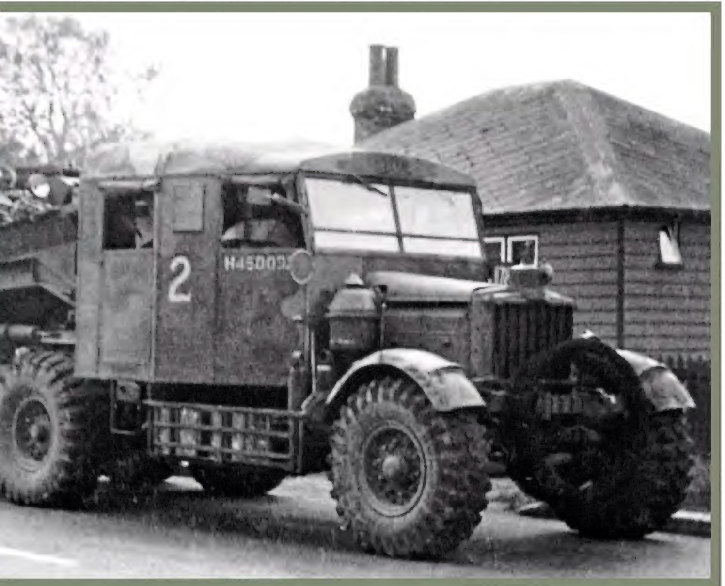
● Early 20-ton Pioneer with the riveted semi-trailer. Like the original 1932 semi-trailer, it was necessary to remove the rear bogie of the semi-trailer to effect loading. Only eight semi-trailers were constructed with this configuration.
