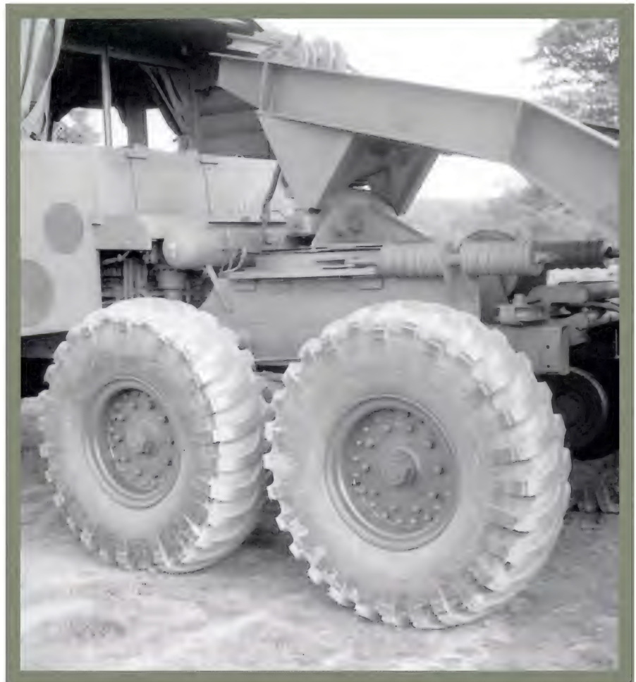
● Close-up view of the turntable of the redesigned 20-ton semi-trailer, with a near-horizontal loading deck. Note the rubber buffers designed to absorb some of the shock loading of moving away from rest with a loaded trailer.
