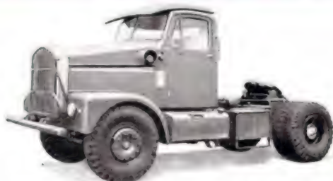
OILFIELDS 12' Wheelbase 4 x 2 Motive Unit. Fitted with fifth wheel turntable for attaching semi-trailers. Load capacity 33,000 lbs.
