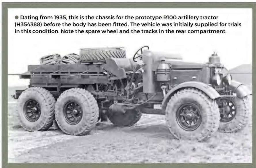
● Early R100 artillery tractor chassis doing what it does best during trials at Watford. Note the tracks enclosing the rear wheels.
