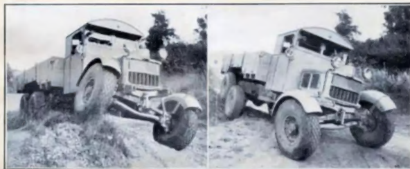
The axle articulation of the Scammell "Pioneer" rigid six-wheeler is one of its special features.
