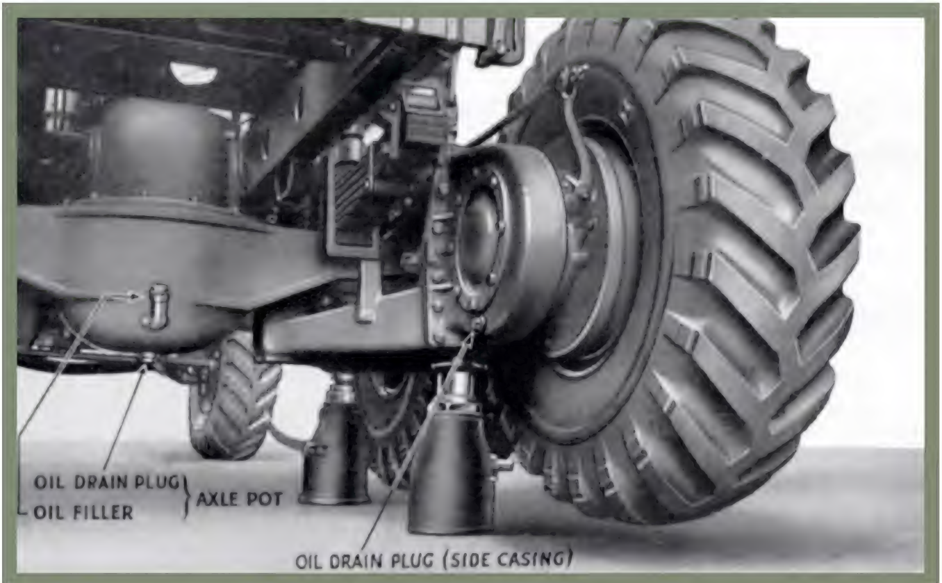
● View under the right-hand rear wheel showing the differential casing, suspension arrangements, and the walking-beam gear case.
