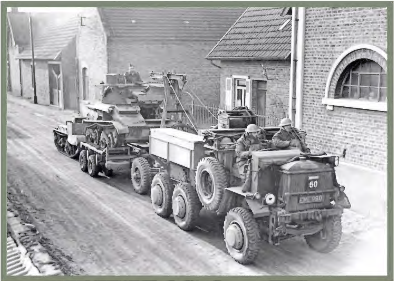
● AEC-FWD R6T artillery tractor coupled to a drawbar trailer via a dummy axle. With a Vickers light tank Mk VIB on the trailer, and a tracked carrier on tow, the outfit is operating as a tank-recovery vehicle. The total weight of the load is in the order of 20,000 lb (9090kg).
