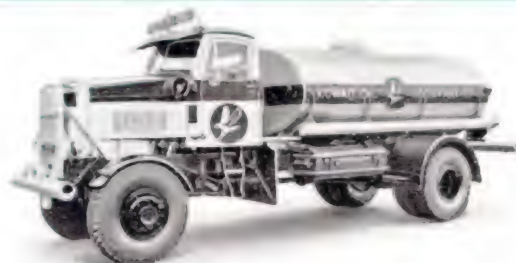
"MOUNTAINEER" 4 wheel drive Tanker for 2,500 Imp. Gals. Petrol/Salt water. Discharge by power driven pump through flowmeter.
