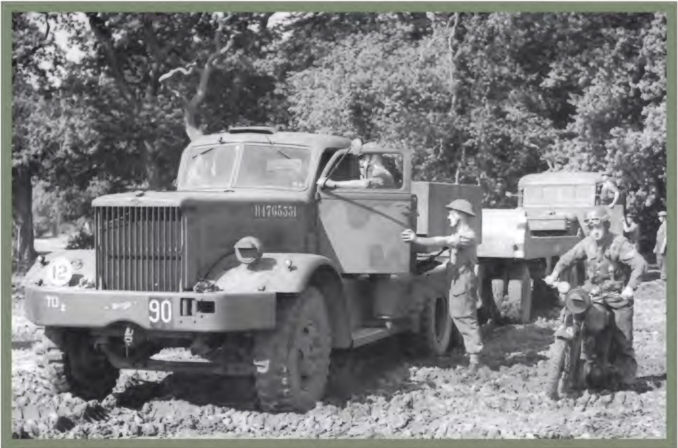
● Well-marked closed-cab Diamond T Model 981 (note the winch fairlead rollers in the front bumper), hitched to a 40-ton Mk II British trailer. The official caption states that the vehicle was taking part in 'a recovery exercise'.
