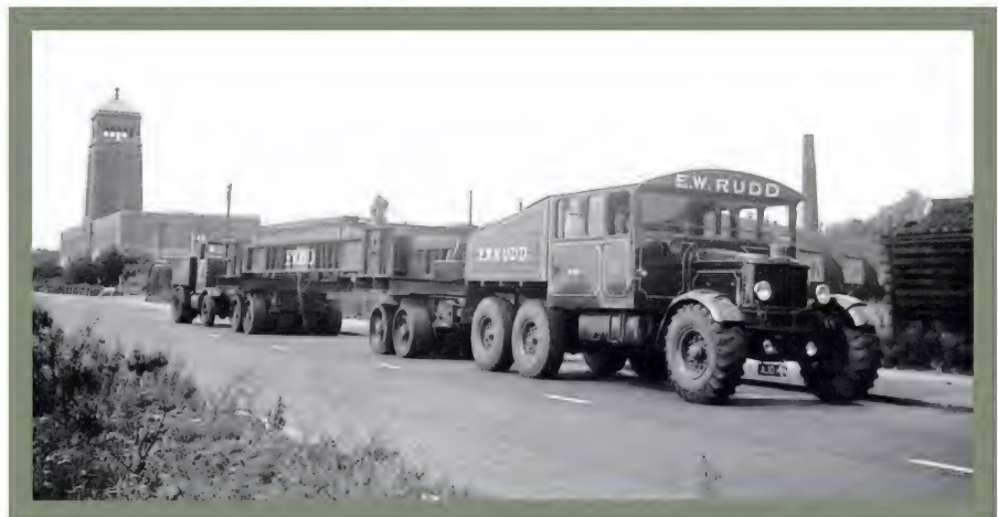
● Another Pioneer 80, this time belonging to EW Rudd. Note how the general appearance of the military Pioneer has been retained despite the cab being increased in width.
