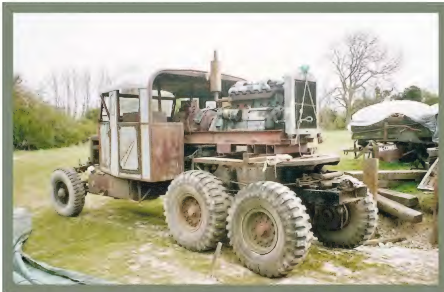
● The script legend on the cab door suggests that this could be another Pioneer that belonged to R Edwards & Sons. Note how the generator set occupies the position previously allotted to the fifth wheel and also protrudes into the cab.
