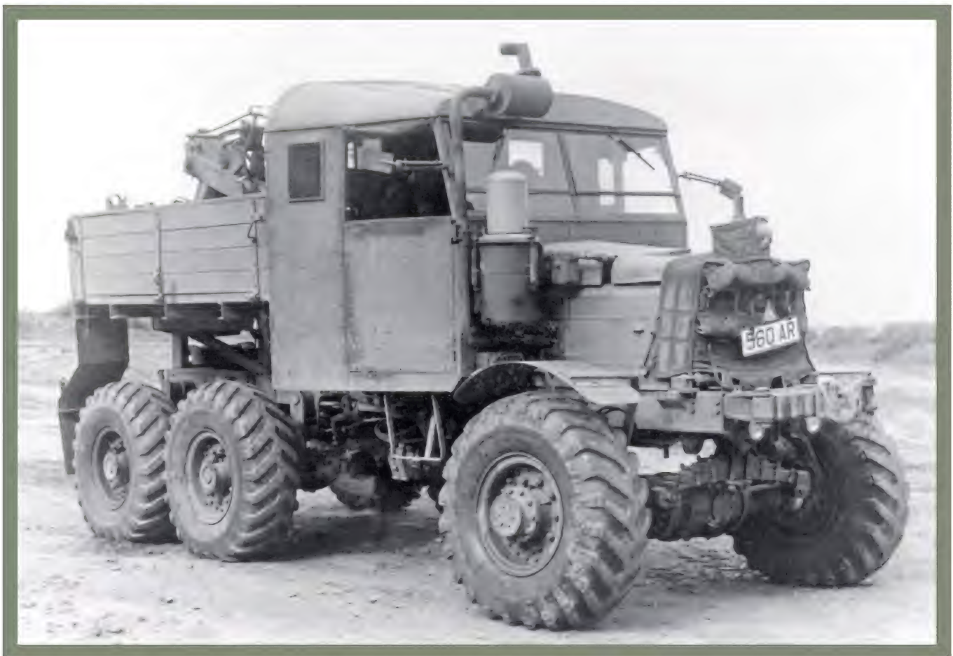
● This somewhat shabby Pioneer SV/2S breakdown-recovery vehicle has been fitted with a Scammell driven front axle. Note, also, the amended height of the engine air intake... clearly deep mud is anticipated!
