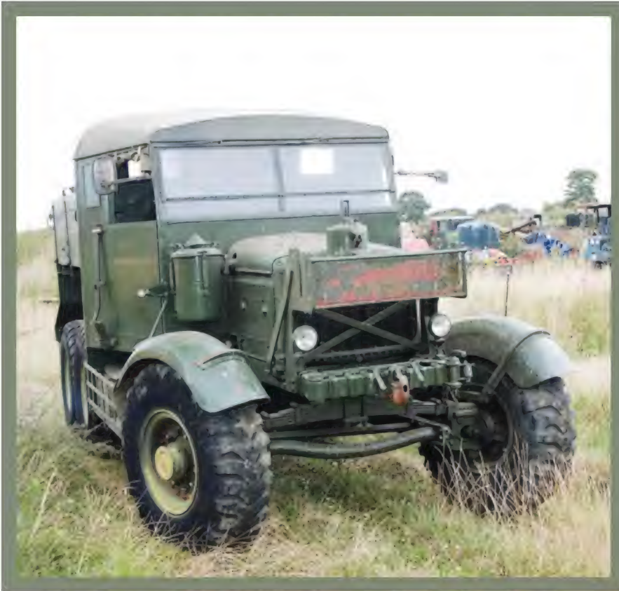
● Privately-owned Pioneer SV/2S breakdown-recovery tractor in typical post-war ex-auction condition, indifferently painted in glossy Deep Bronze Green.
