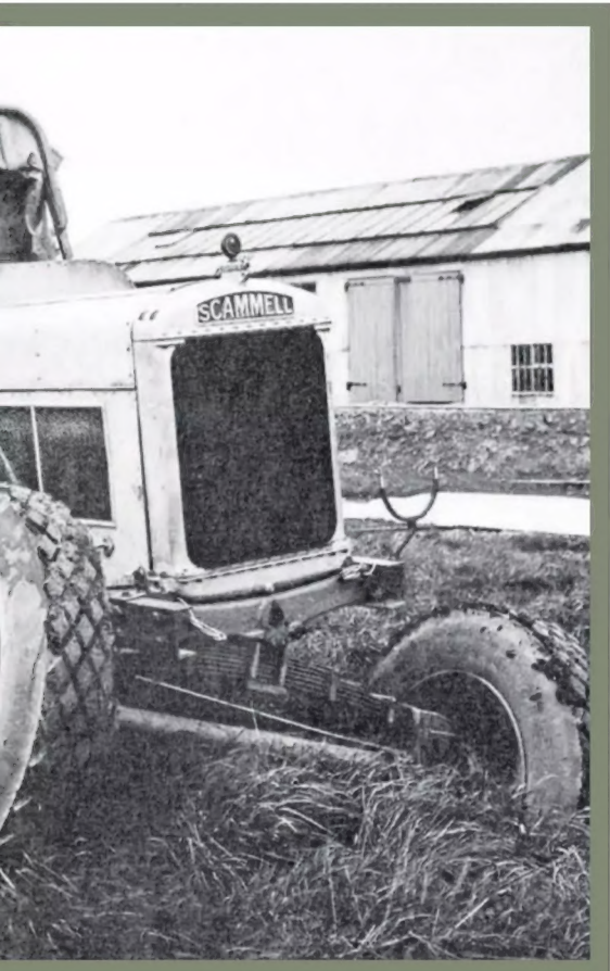
● (BELOW) Photographed in June 1927, the Pioneer prototype, although still not yet identified as such, exhibits the major features that would ultimately define the Pioneer... the walking beam gear-cases at the rear, and the pivoting front axle. The distinctive cast radiator surround has yet to appear.
