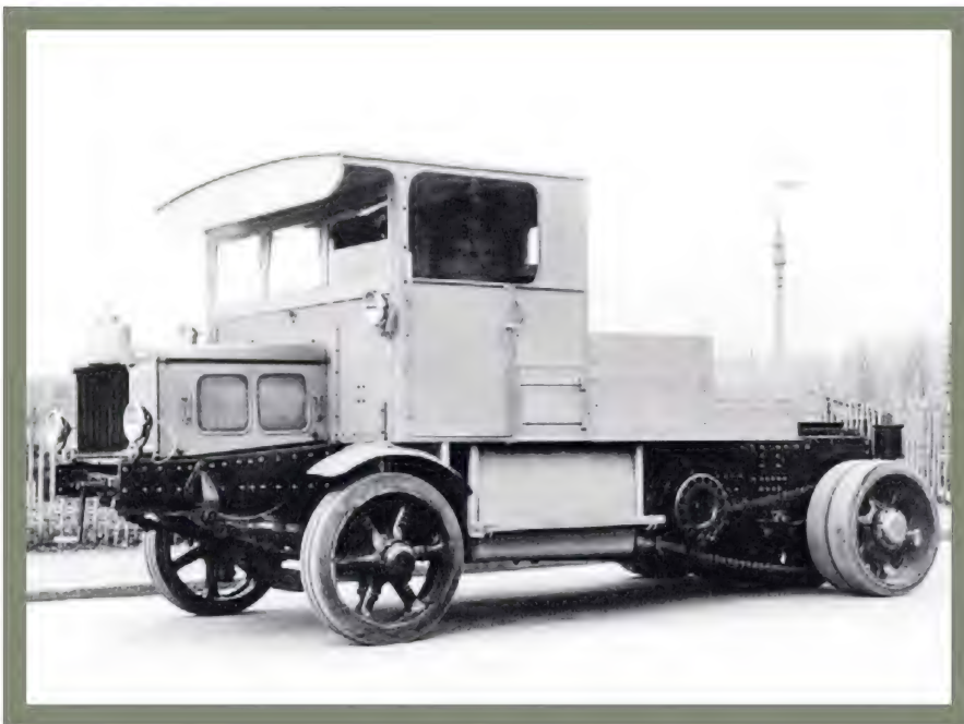
● The '100-tonner' was constructed around a unique riveted box-frame design and was originally powered by a 7-litre Scammell four-cylinder engine, although this was eventually replaced by a Gardner 6LW diesel unit. This is the first of the two tractors to be constructed.
