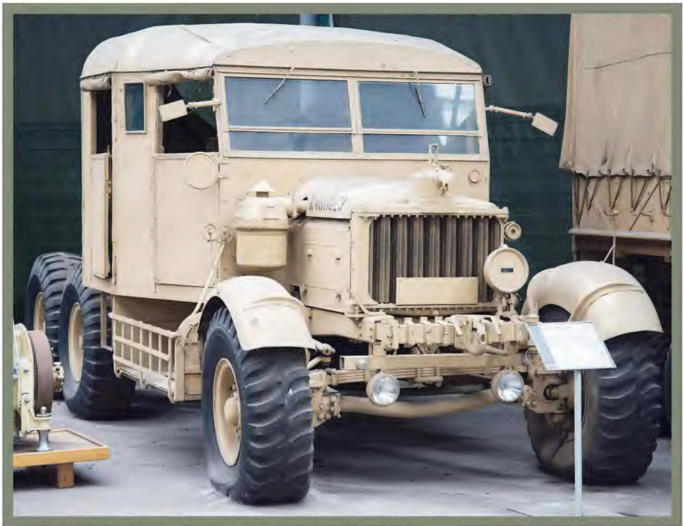
● Looking a little tired and cobwebby around the wheels, this tank transporter was photographed at the REME Museum. The side lights and the lower headlights are later additions.
