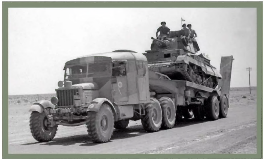
● Late-model 30-ton Pioneer with the modified trailer deck that has been dropped down on either side of the swan neck. The load is a Cruiser Mk II tank. Note the dazzle-pattern camouflage applied to the tractor, typical of vehicles in the North African theatre, and consisting of a base colour of light-stone, over which are applied 'shadows' of dark grey and blue.
