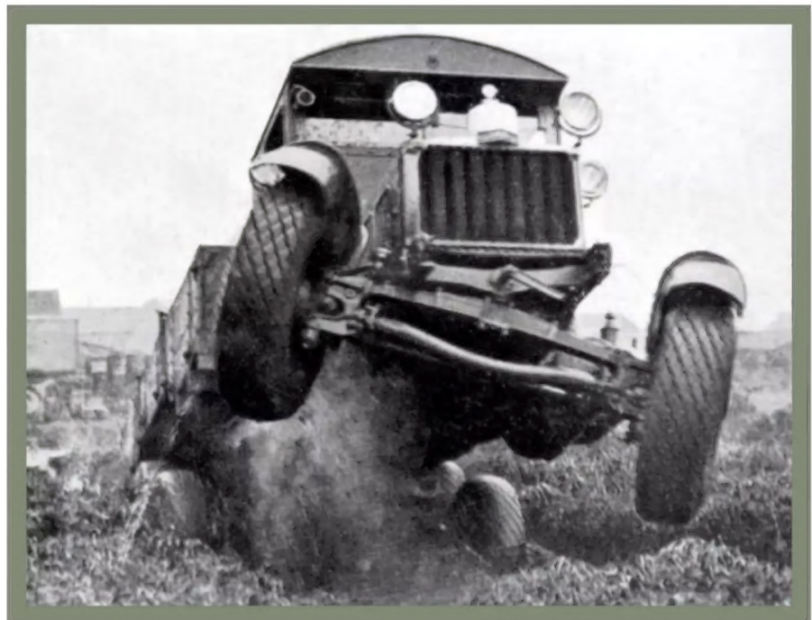
● With the pivoted front axle at full deflection, and the front wheels apparently clawing for purchase in mid-air, an early Pioneer shows just what it was made of... all of this without front wheel drive, remember!
