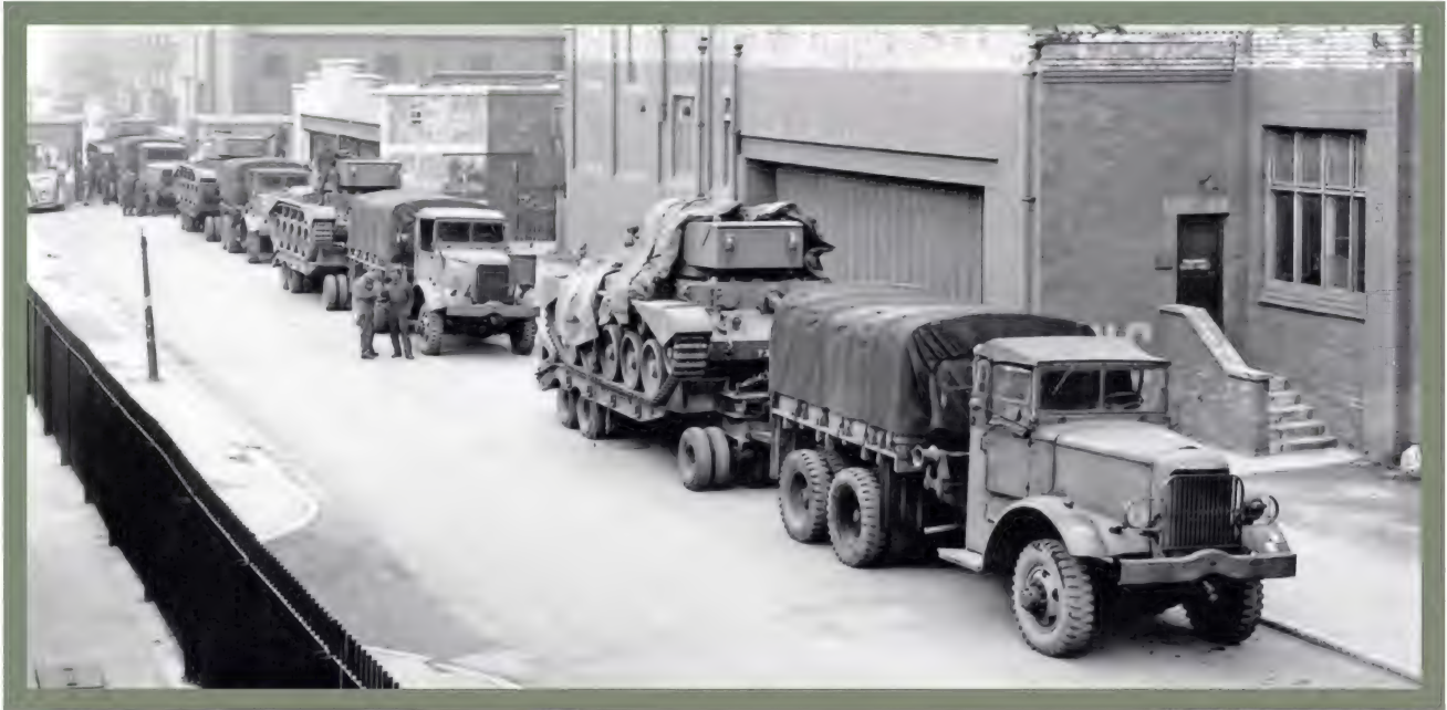
● Photographed at the Leyland works in 1944, a convoy of four Mack NM5 tractors, with drawbar trailers, line up to deliver newly-manufactured A34 Cromwell tanks. The combat weight of a Cromwell was 78,800 lb (35818kg), rather more than could be handled by even a 30-ton Pioneer.
