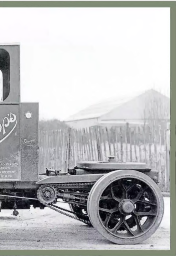
● (BELOW) Photographed in June 1927, the Pioneer prototype, although still not yet identified as such, exhibits the major features that would ultimately define the Pioneer... the walking beam gear-cases at the rear, and the pivoting front axle. The distinctive cast radiator surround has yet to appear.
