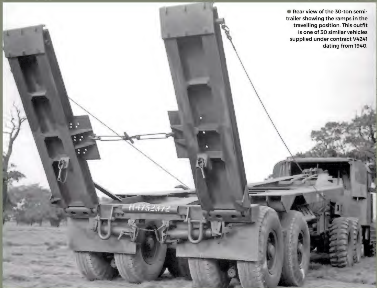
● The rear strainers are adjusted until the chains are tight enough to prevent the tank moving on the semi-trailer during transport. Note the locking handles used to secure the ramps in the upright position.
