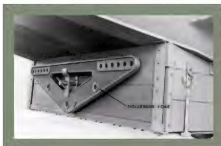
● The Hollebone yoke in its stowed position under the semi-trailer.
