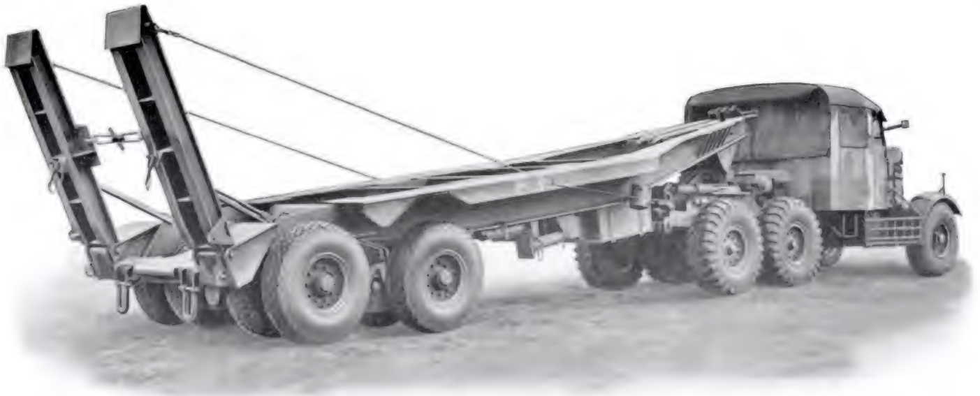
● Rear three-quarter view of the 30-ton Pioneer with the original steeply sloping deck. Note the centre-of-gravity markings on the sides of the semi-trailer.
