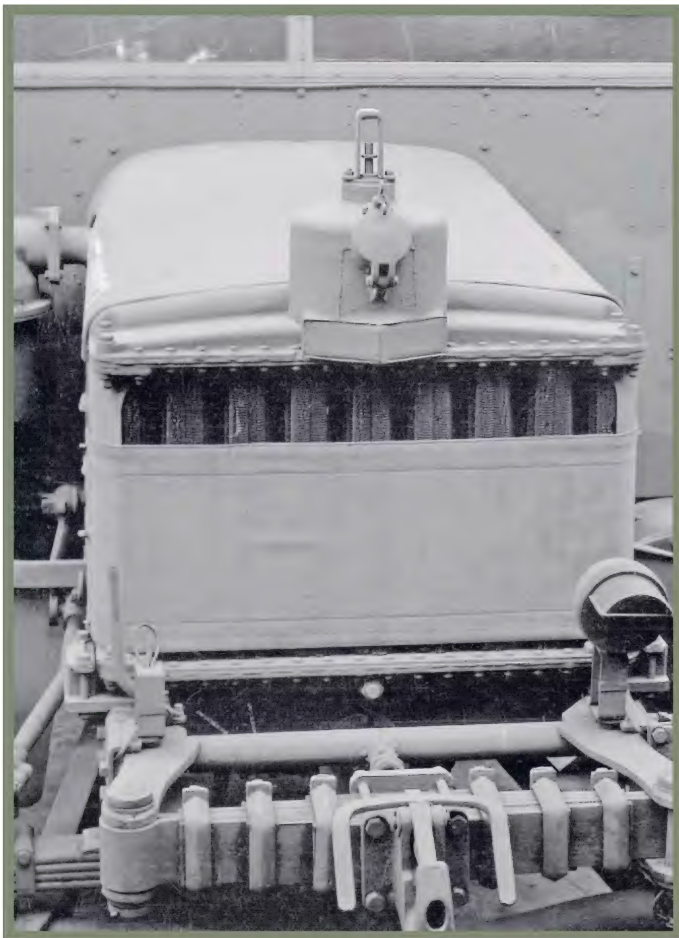
● View of the front end of the Pioneer, showing the sprung tow hook, radiator blind, blackout light, and the radiator, with its distinctive 'teapot'. Note how the radiator now lacks the 'Scammell' name which, on early production vehicles, was cast into the plinth supporting the 'teapot' itself.
